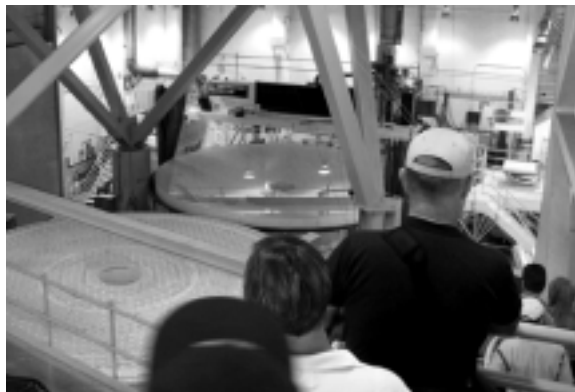
A pair of 6.5 meter mirrors are being produced. One mirror is nearly completed. The closer mirror is actually upside down at this time. The mirror construction lab is located under the university's football stadium because the large concrete structure adds stability.
