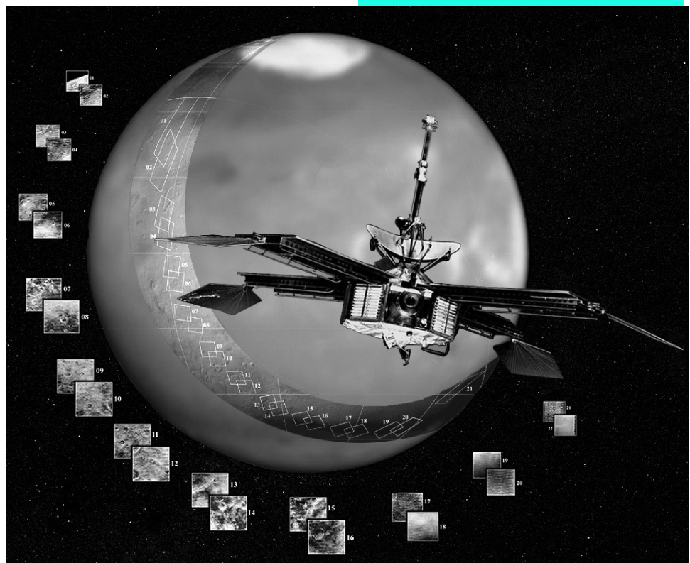
In this poster art of Mariner 4, you can see the parabolic reflector atop the spacecraft bus. Like the reflector inside a flashlight, it sends a beam of electromagnetic energy in a particular direction. Credit: NASA/JPL/Corby Waste.
