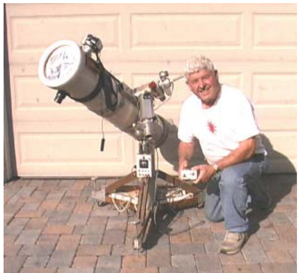
Photo #2. The author with his home-built, 8-inch Newtonian reflector (f/5.6) used for the 2006 transit.
