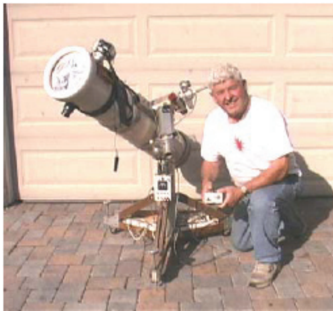
The author with his home-built, 8-inch Newtonian reflector (f/5.6) used for the 2006 transit. Photo courtesy of Ernie Piini.
