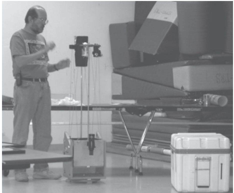
Rob Hawley demonstrates his string Dobsonian which he successfully used on his trip to Costa Rica. Both string Dobs are 8" f/6 and based on a design by Charles Wickes. Photos courtesy of Mary Kohlmeier.
